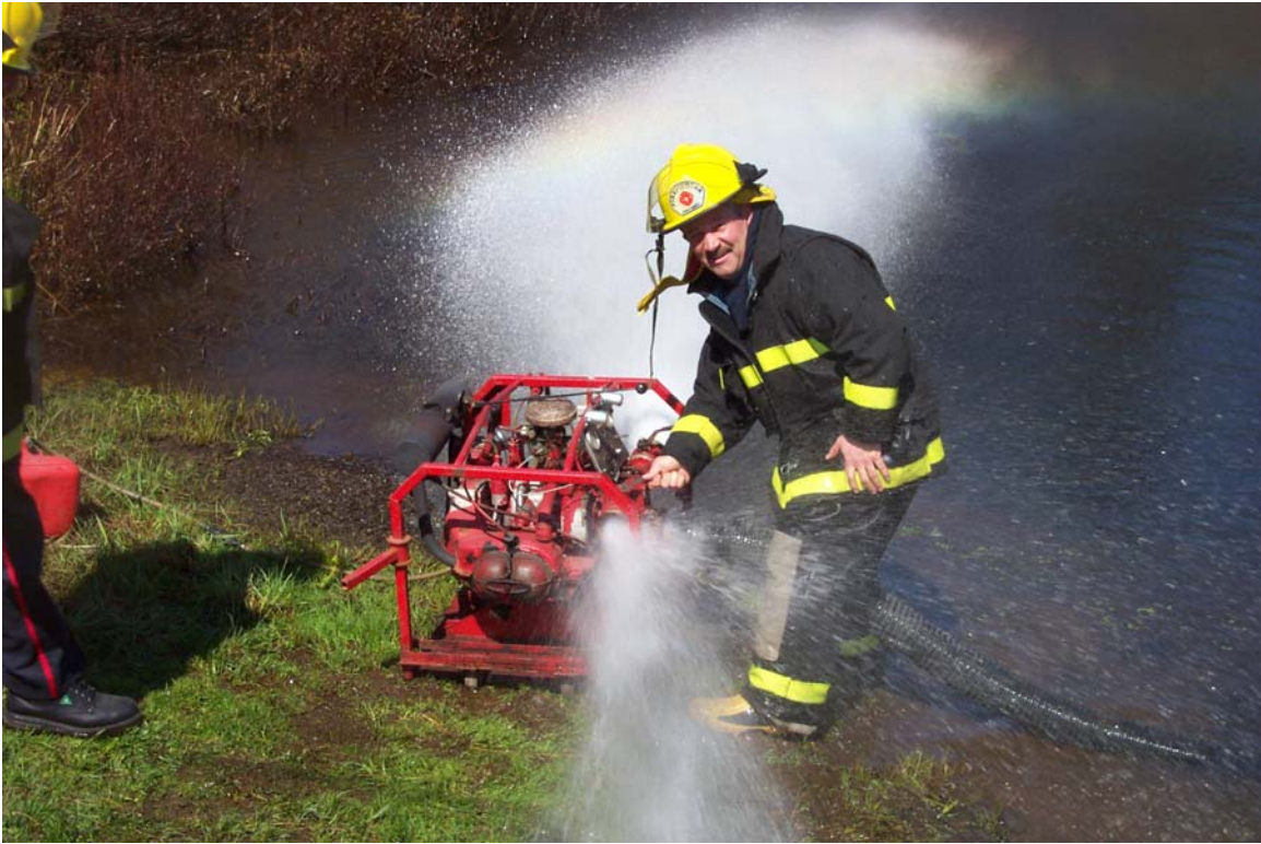
Photo: Conception Bay South Firefighter Kevin Whelan runs a portable firefighting pump during a recent training session in preparation for the 2006 forest fire season.
